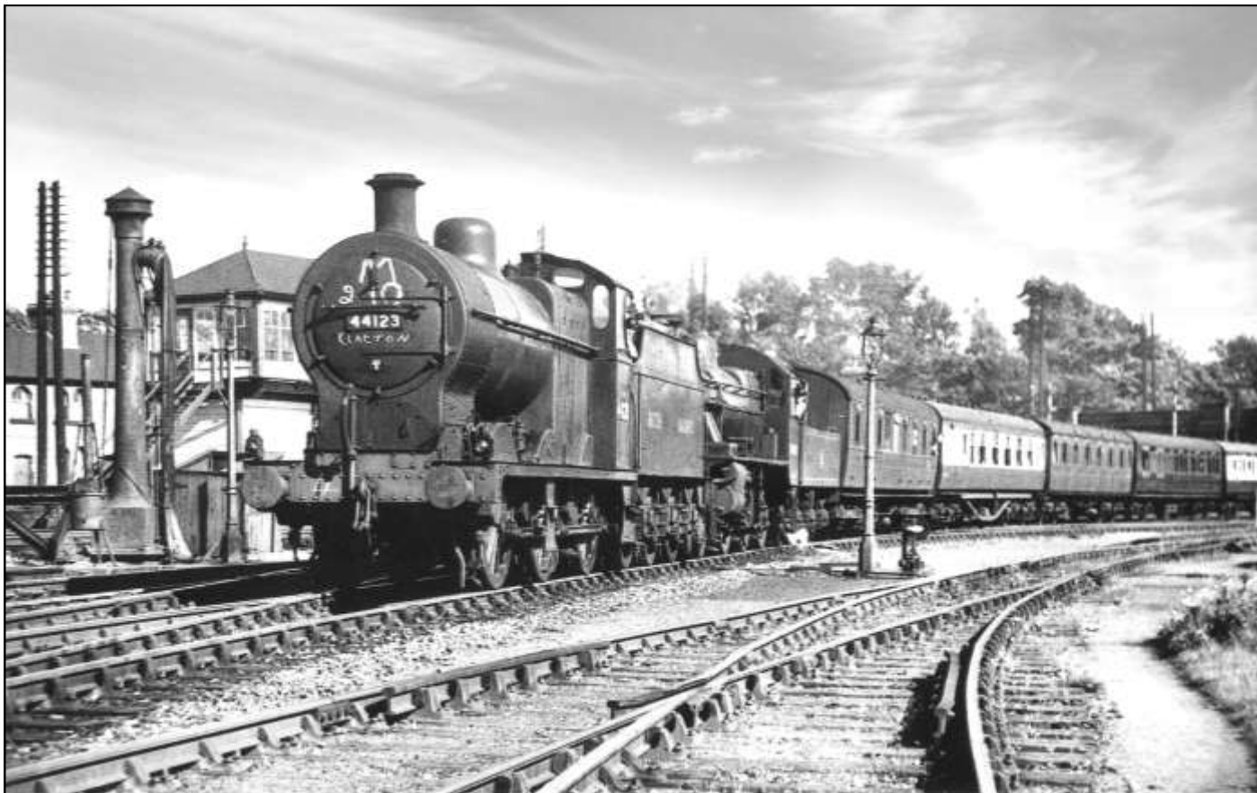
A double-headed excursion train headed by steam engine number 44123, a 0-6-0 class 4F locomotive, just passing the Wigston South Junction signal box as it pulls out of Wigston Magna Station.
