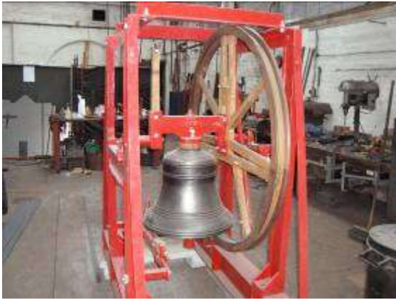
A testing frame, the rope is controlled . by the large wheel to the right.
