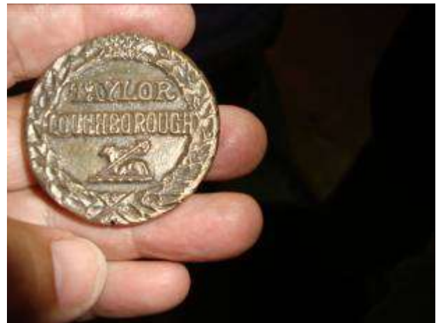
An embossing die. All bells are embossed with company stamp, date cast, order number and pattern number.
